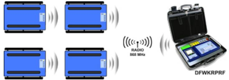
Example of application with 4 wireless platforms and DFWKRPRF indicator for the reading and printing of the weight through a remote indicator.
